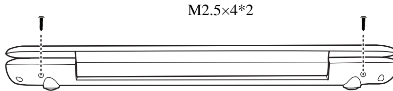
Figure 4.28 Removing the screws from the rear of the laptop
